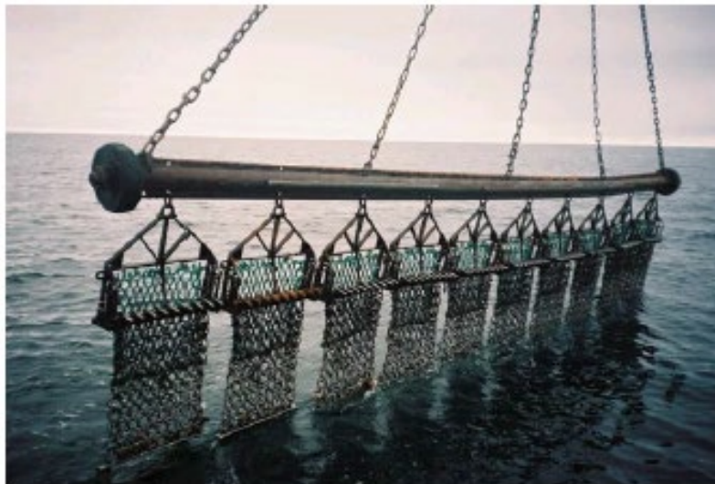
Figure 12-3A toothed, spring-loaded dredge used for Scallop fishing
